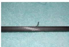
The other ways to hold guides are with tape or rubber bands. Tape works if you have your guide position set and are ready to wrap. Use 1/8" or 1/4" tape strips to hold the guide on the blank. Position the tape or the band near the guide frame so you can wrap the foot of the guide with thread to hold it, and then remove the tape or the bands. Just cut the band or unwrap the tape when you run out of room.
