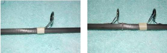
Good sources of rubber bands are the ones used in braces or strips of surgical tubing cut to width. The surgical tubing is better for larger guides as you can cut it wider as needed.
