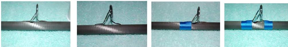
The guide with one wrap above has been prepped properly. Note the smooth transition from the blank to the guide foot. The guide with both feet wrapped above was not prepped. Note the bumps at the end of the guide foot. This will cause a finish crack over time.
