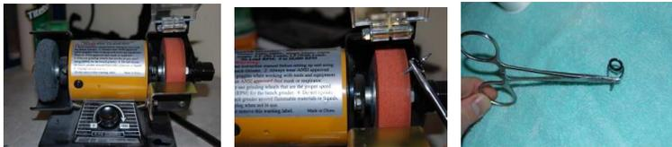
Once the desired shape is achieved, use the fiber wheel to polish and smooth both the underside and the top side of the guide. In most cases, the guide will be resting on the blank so if the foot is not flat, or there are burrs on the bottom, it could create a wear point for the blank to fail. Having personal experience here, I can tell you it will happen. Also ensure that the feet are bent so it all lays flat on the blank. Note the prepped and unprepped pictures below.
