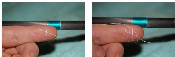
Hold the wrap against the blank with your right index finger. Grab the tag end to the right with your thumb and second finger. Pull out your left index finger from the wrap and grab the left tag end. Tighten both tag ends at the same time. The wraps will want to cross over each other and usually this isn't a huge deal if you burnish after. But if you get good at this, you can tighten the knot without crossovers.
