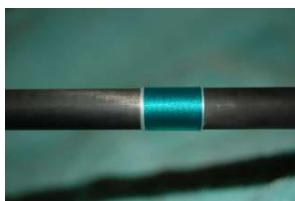
If you have trouble with the band slipping after it's done, then you can carefully apply a drop of color preserver to the crossover knot so it holds. This is the most helpful method when using metallics for trim.
