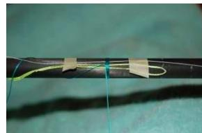
Begin wrapping the trim band and put on the number of turns you want for the trim. Untape the tie-off loop and pull through the tag end under the main wrap. Trim the ends and continue the main wrap.
