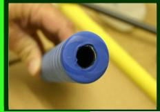
Hold the heated ends until they cool. The ends should be flat and conform to the face of the grip
