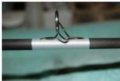
Some builders apply a coat of finish to the under wrap before wrapping the guides, some just use color preserver, some don't do either. If you've used A thread for the under wrap and plan on using A thread for the guide wrap, you'll have problems with the over wrap thread lining up in the grooves of the under wrap and may create some gaps. D thread for the over wraps will cause less of an issue. The easiest way to proceed is to apply a coat of finish to the under wrap before wrapping the guide.
