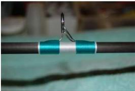
Measuring tools can be beneficial in ensuring you get the guide and wraps centered on the under wrap. The visual contrast of the under wrap will magnify any difference in length between the wraps on either foot so take a minute to ensure you have the guide in the right place on the over wrap and the resulting guide wraps will be of equal length.
